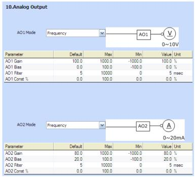
Set the parameters corresponding to Analog Output.
