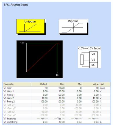
Set the parameters corresponding to V1 Analog Input.
