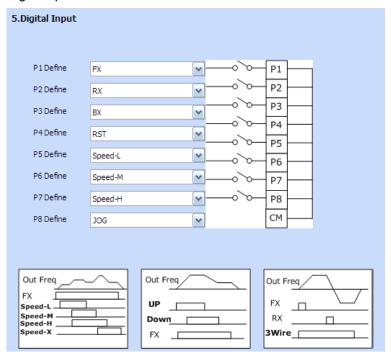
Set the parameters corresponding to Digital Input.
